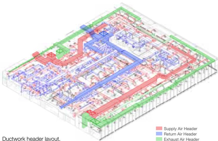
Ductwork header layout.
