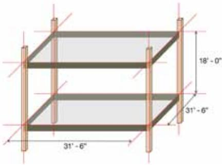
The universal grid-planning module comprises an optimum set of vertical and horizontal dimensions for the structural bay of a building.
